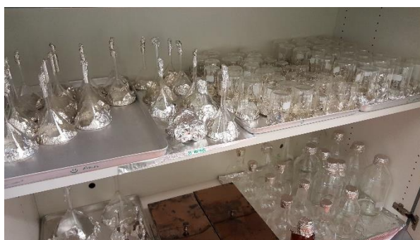
Figure 2. Storage of glassware sealed with aluminium foil to keep out dust.
